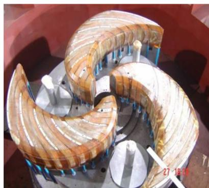
Figure 5: The trim coils are mounted on the pole tip and then vacuum impregnated with epoxy resin.
