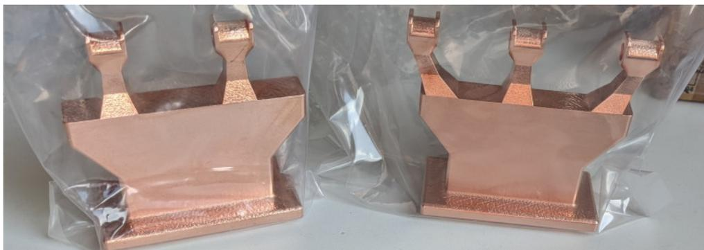
Figure 6: First iteration of AM stainless-steel IH-structures after polishing and galvanic copper-plating.
