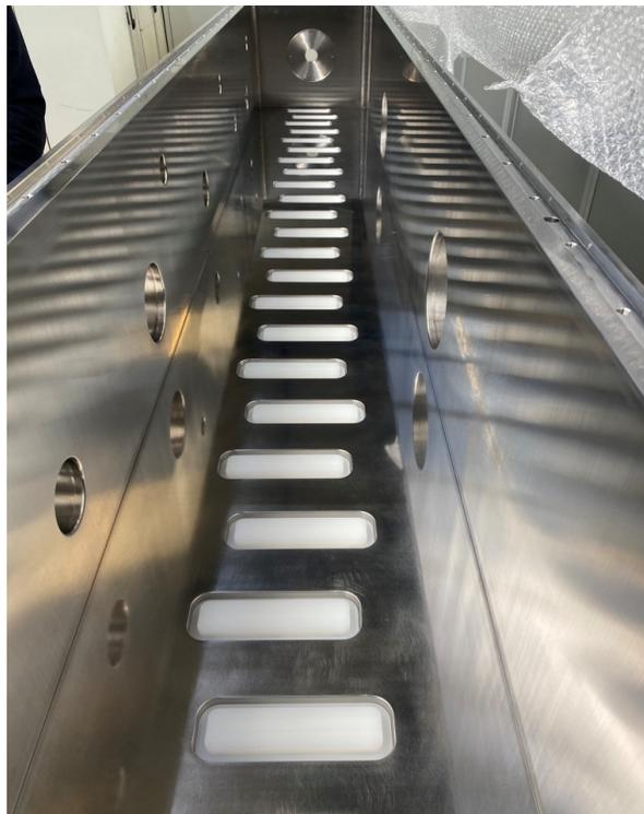
Figure 3: RFQ stainless steel tank with cut outs for the stems.
