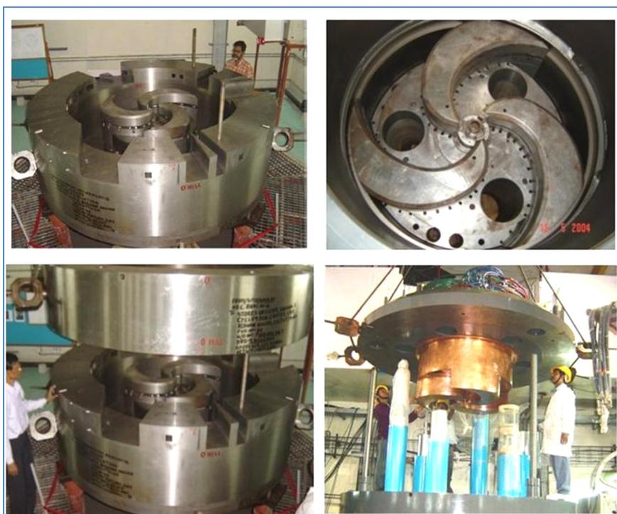
Figure 3: Different parts of iron frame of the magnet: lower half of the magnet (at top-left), three spiral hills (at top-right), return yoke ring (at bottom-left), upper half of the magnet (at bottom-right).
