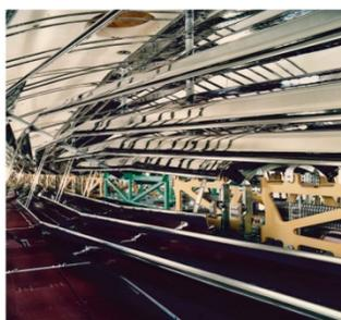
Figure 6: The Vivitron, a 20 MV large tandem. View on the terminal, longitudinal structure and intermediate polarized porticos distributed radially.
