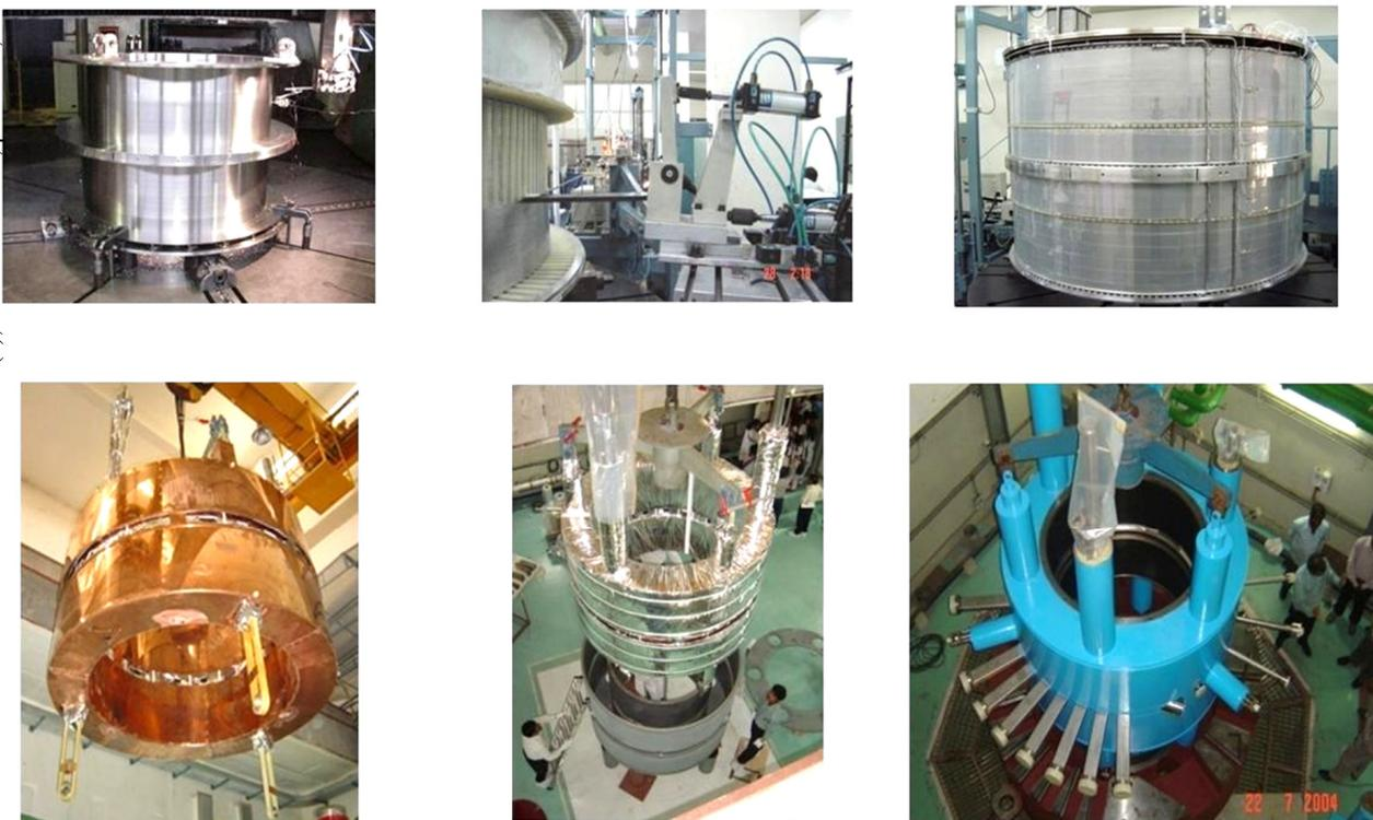
Figure 4: Different parts of cryostat and coil assembly: bobbin made of Stainless Steel (at top-left), Coil-winding machine (at top-middle), superconducting primary coils (at top-right), Copper made liquid nitrogen cooled radiation shield (at bottom-left), MLI wrapped coil plus shield being inserted into the cryostat vacuum chamber made of magnetic steel (at bottom middle), Coil tank with its radial inserts being installed on magnet (at bottom-right).
