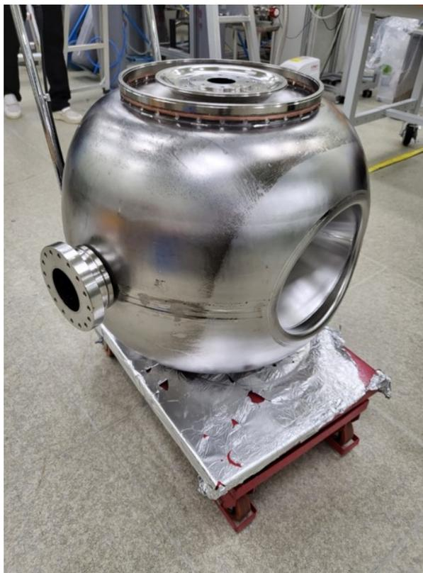
Figure 2: Fabricated SSR2 Bare Cavity.
