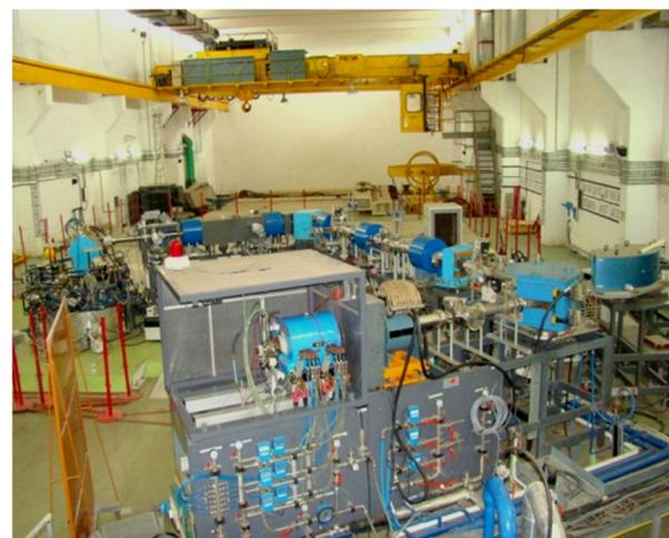
Figure 2: 14GHz ECR ion source and injection beam line.
