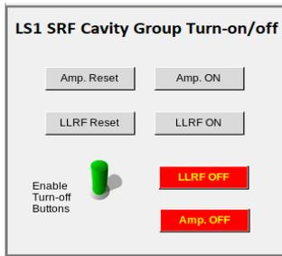
Figure 6: OPI for turning on/off LS1 SRF cavities.
