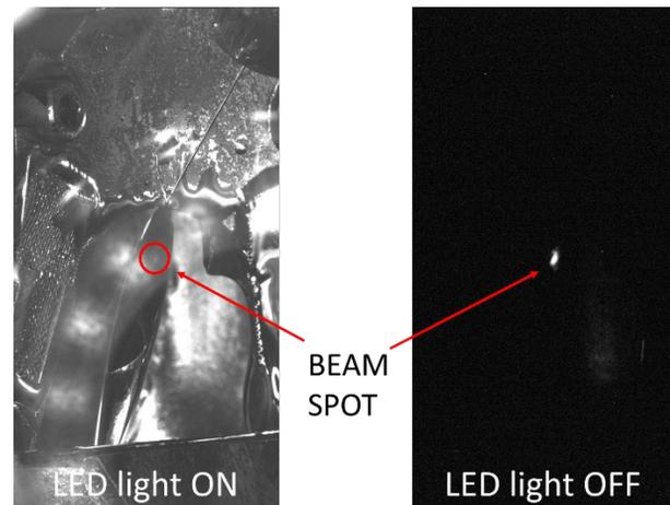
Figure 8: Beam spot on the LLCS during the high-intensity irradiation test. The LED light was turned off on the right photo to take a clear beam spot.
