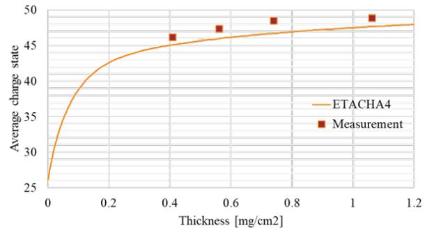
(a) Average charge states of xenon beam stripped by lithium.
