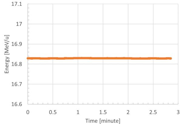
Figure 7: <sup>36</sup>Ar beam energy after the lithium stripper during the high-intensity irradiation test (peak intensity 12 particle μA, peak beam power 7400 W (average 400 W, duty cycle 5.4%), peak power loss 50 W (volumetric power deposition 6 MW/cm<sup>3</sup>).
