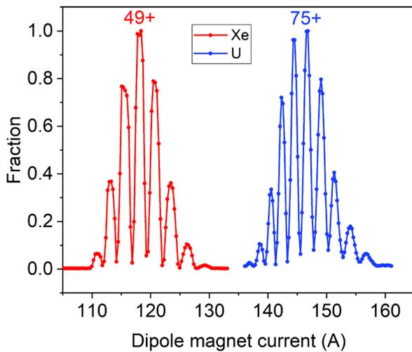
Figure 5: Xenon (red) and uranium (blue) charge state distributions after the liquid lithium stripper. The thickness is 1.05 mg/cm<sup>2</sup> for the xenon beam and 1.40 mg/cm<sup>2</sup> for the uranium beam.
