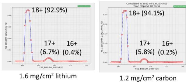
Figure 6: Charge state distributions of 20 MeV/u argon beam after the LLCS and carbon foil stripper. Thickness was 1.6 mg/cm<sup>2</sup> and 1.2 mg/cm<sup>2</sup> for the lithium and the carbon, respectively.
