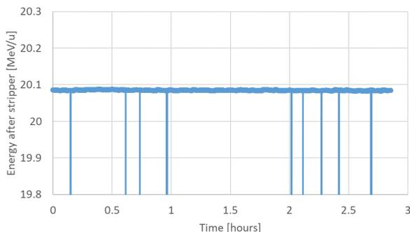
Figure 9:  $^{48}\text{Ca}$  beam energy after the lithium stripper. At downward spikes the beam was tripped.
