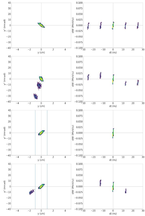
Figure 7:  $Y$ - $Y'$  (left) and longitudinal (right) beam snapshots simulated by TRACK: before the chopper, after the chopper, before the beam dump, and after the beam dump (vertical lines represent aperture size).
