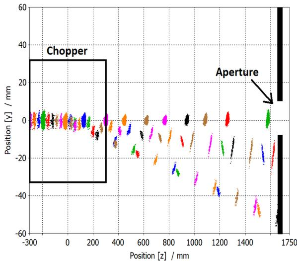
Figure 6: CST Studio simulation of the trajectory of bunches through the chopper, drift space, and the aperture.
