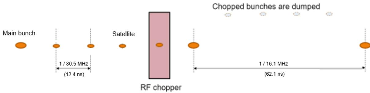
Figure 3: Bunch structure before and after the RF chopper system.
