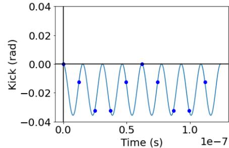
Figure 5: Average bunch deflection in the chopper due to the RF electric field combined with the static magnetic field provided by the chopper dipole overlaid onto a 64.4 MHz waveform.
