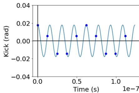
Figure 4: Average bunch deflection in the chopper due to the RF electric field overlaid onto a 64.4 MHz waveform.
