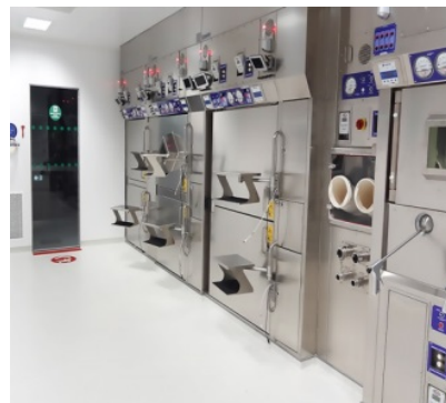
Figure 9: Hot cell of CYRCé facility used for radiobiology, hadron therapy and medical imaging research at IPHC. Equipment is adapted to the manipulation of cells, samples, hot targets, radionuclides and other components.
