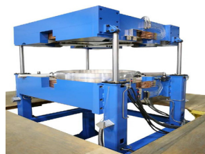
Figure 7: TR24 cyclotron with open structure. Coils, magnet and vacuum chamber are removed.
