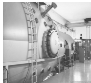
Figure 5: The new MP VDG tandem accelerator commissioned at 9 MV in 1972 and upgraded at 18 MV.
