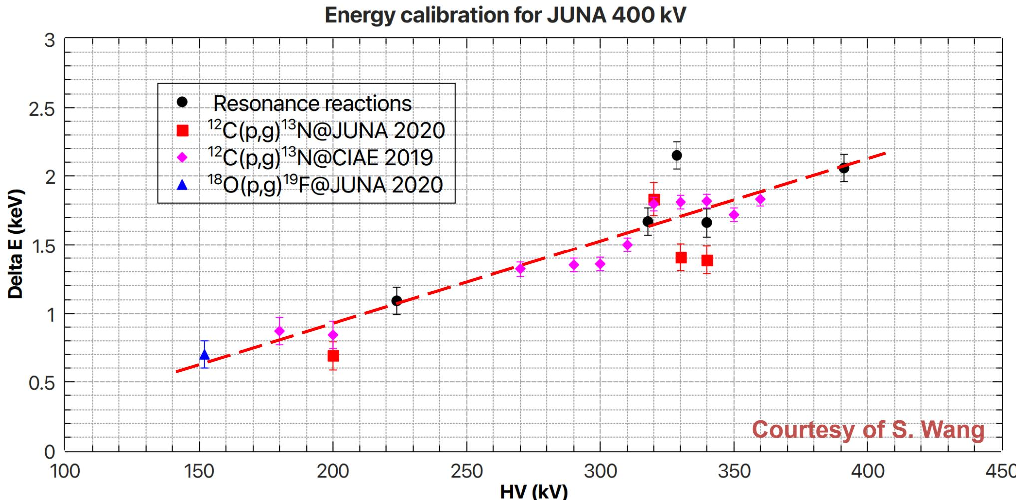
Linear dependence of the observed energy deviation vs. applied voltage
