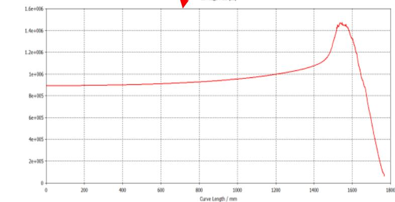
Max electric field <15 kV/cm
