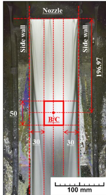
Figure 8. Appearance of the Li target under the IFMIF conditions (250 °C, 15 m s<sup>-1</sup>, 10<sup>-3</sup> Pa).
