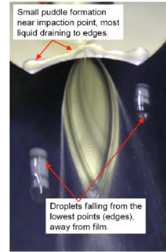
Figure 43 – Pictures of old and new deflectors in operation.
