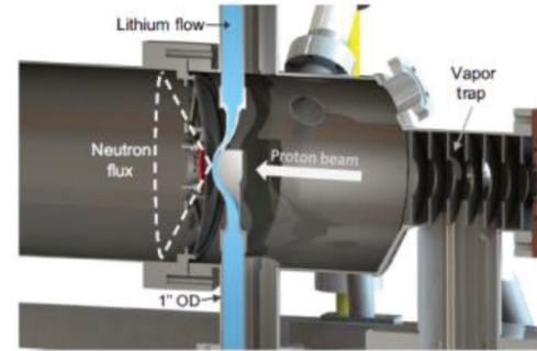
FIGURE 3. LiLiT target, for details see [5]. The sample to be irradiated by the neutrons can be placed at about 1 cm from the target (the red line) and is exposed there to neutron flux of about  $2 \times 10^{10}$  n/s/cm<sup>2</sup>/mA
