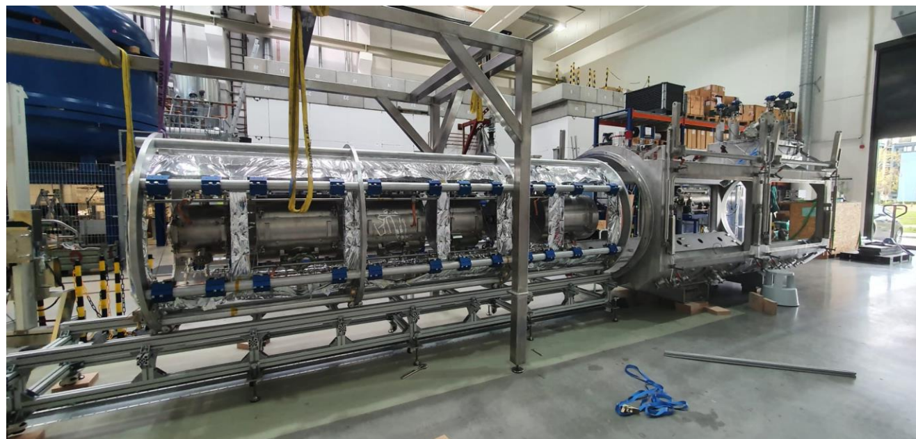
Cold string assembly
