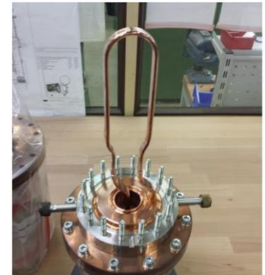
the coupling of the cavity could not be significantly improved by exchange of coupling loop in 2021
