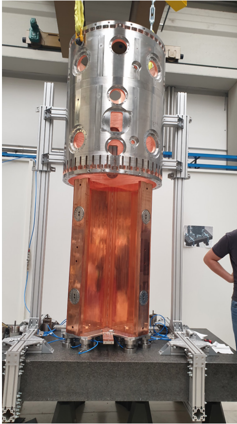
Initial positioning of the tank vs electrodes in vertical position
