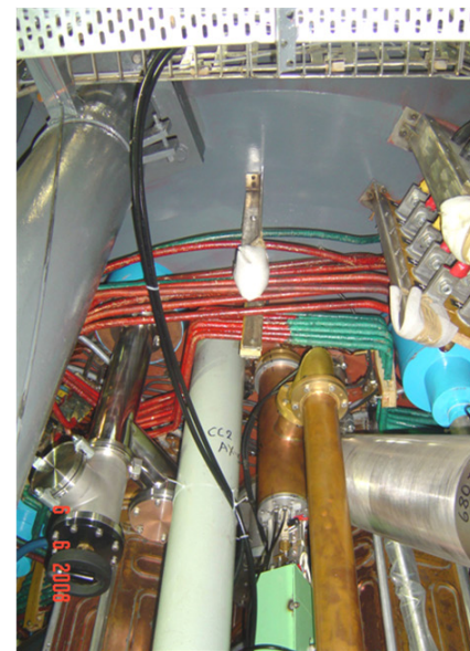
RF Amplifier feeding power to the cavity through Coupling Capacitor
