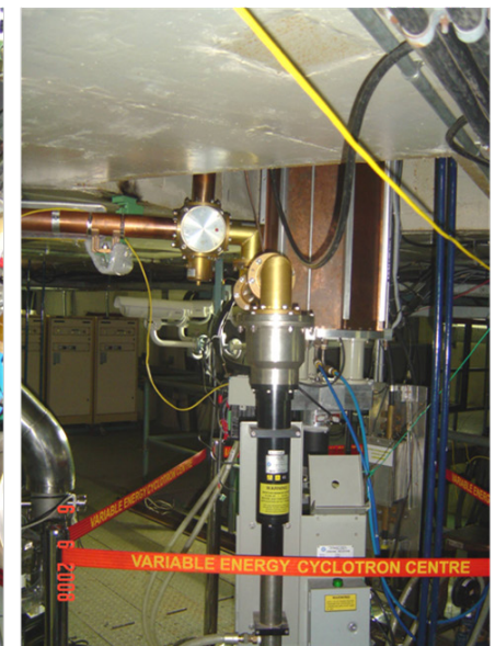
RF Amplifier feeding power to the cavity through Coupling Capacitor
