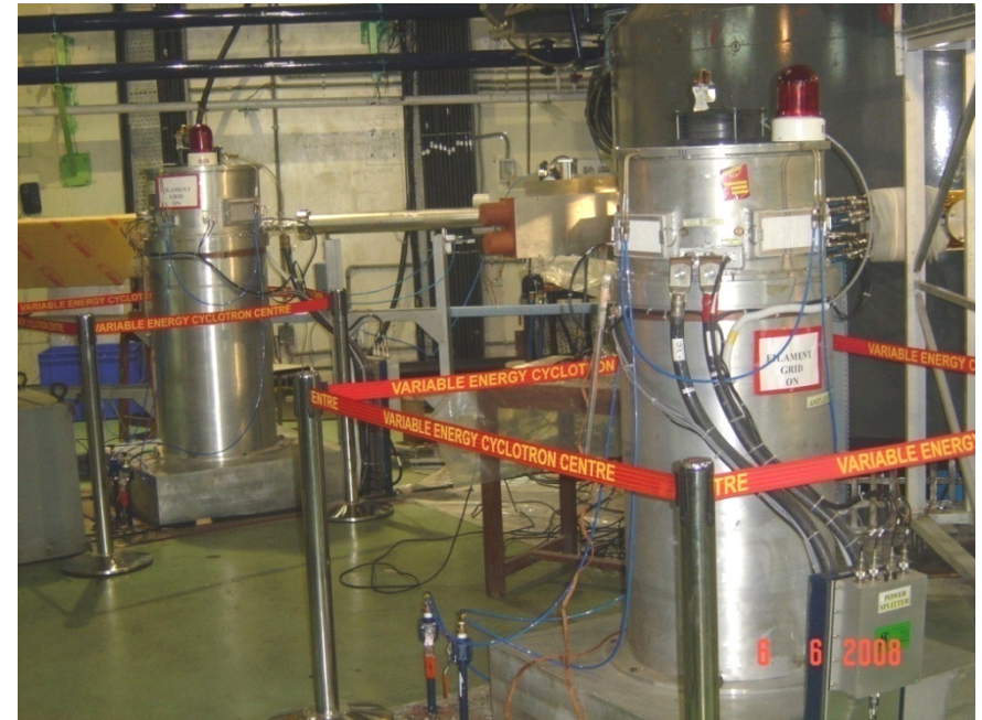
RF Amplifier feeding power to the cavity through Coupling Capacitor
