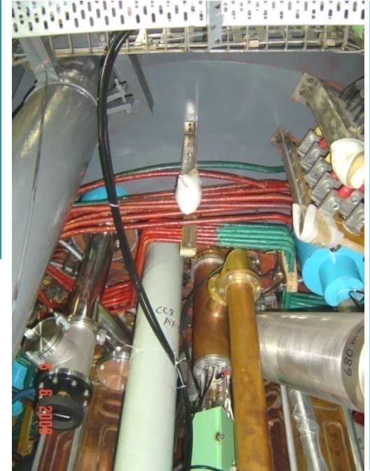
RF Power feeding to main cavity via Coupler
