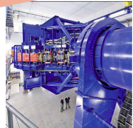
HIT C-ion gantry (600 tons)
